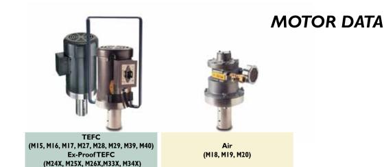
Power Electrical Certification Model Description Туре RPM Requirements HP TEFC (Totally Enclosed Fan Cooled), IP54 Motors MI5 3,450 MI6 230-460VAC/60 Hz 2 1,725 MI7 1,725 3 M27 3,450 Т Continuous duty, 12 ft. (3.5 m) cord. Induction M28 115-230VAC/60 Hz 2 1,725 M29 1,725 3 M39 2,900 220-380-440VAC/50-60 Hz M40 2 1,450 **Explosion Proof Motors**
