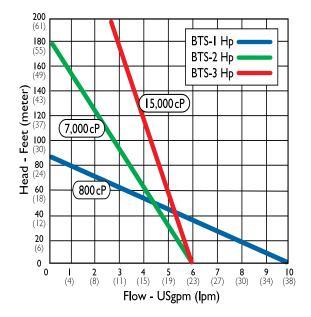
\*When pumping flammables or combustibles, use explosion proof electric or air drive motors on stainless steel tubes with static protection kit. \*\*Performance will vary with changes in fluid viscosity and specific gravity. All testing done at 60 Hz. **Contact factory for 50 Hz data.** BT Series is not recommended for pumping thin water-like fluids.
